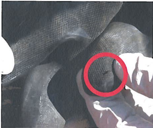
Small hole (highlighted in red) leads to serious injury from HF exposure
