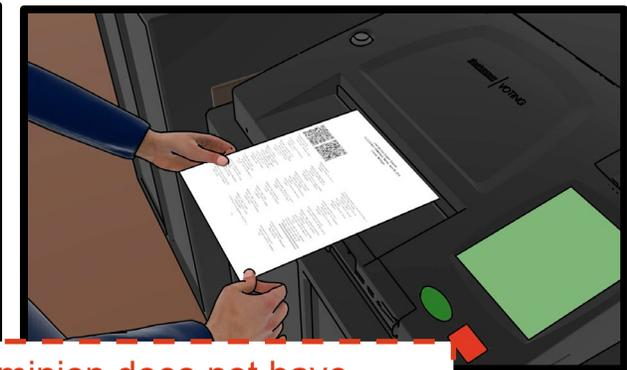
Voters insert their paper ballot into the tabulator, which drops into a secure box. These paper ballots provide a paper trail for later reference, if necessary.
